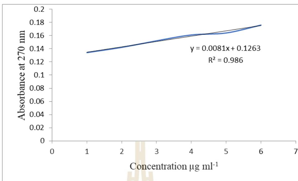
**Attached figure 4** Standard curve of protein concentration at the absorbance 270 nm.
