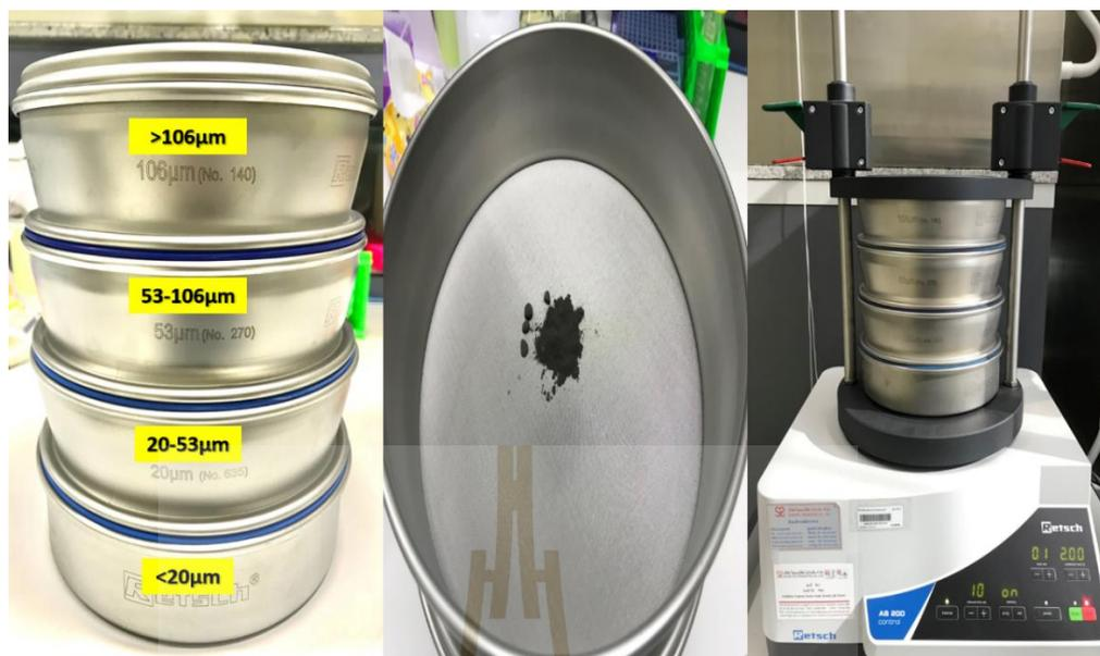
**Figure 3.5** Sieve screen process.
