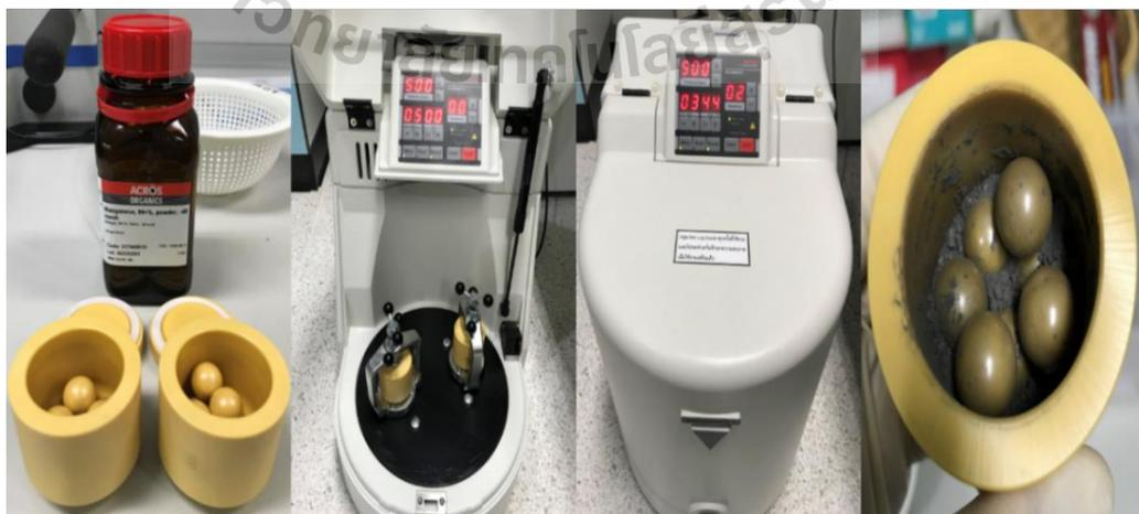
**Figure 3.4** Planetary mill process.
