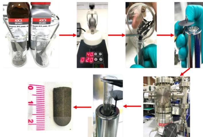
**Figure 3.3** The procedure for the synthesis of MnBi magnets starts with mixing Mn and Bi powders.
