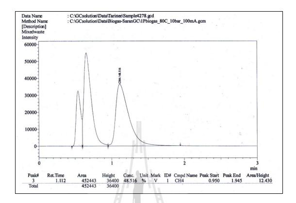
Figure 4.2 Chromatogram and report of methane and nitrogen analyzed by the gas
