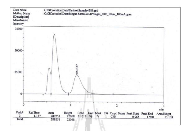
Figure 4.4 Chromatogram and report of methane and nitrogen analyzed by the gas
