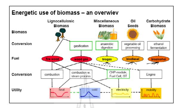
Figure 2.3 Biomass and energy used (after Omolola, 2007)
