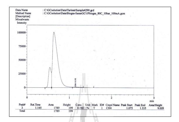
Figure 4.5 Chromatogram and report of methane and nitrogen analyzed by the gas
