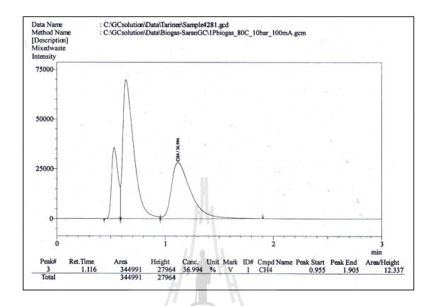
Figure 4.3 Chromatogram and report of methane and nitrogen analyzed by the gas
