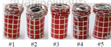
Fig 4 The deformation shape of thin-walled tubes specimen from the experiment
