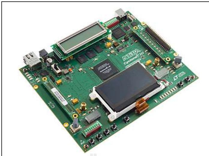
**Figure 6.2** Photograph of Altera cyclone III development board.
