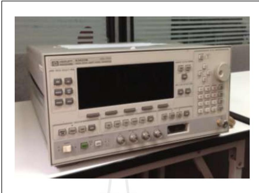
**Figure 6.12** Photograph of Hewlett Packard 83620B signal generator.
