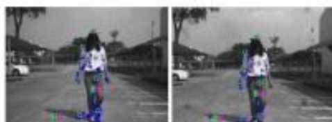
Figure 6. Example results of optical flow feature matching from stereo camera with 5-cm distance between both camera.
