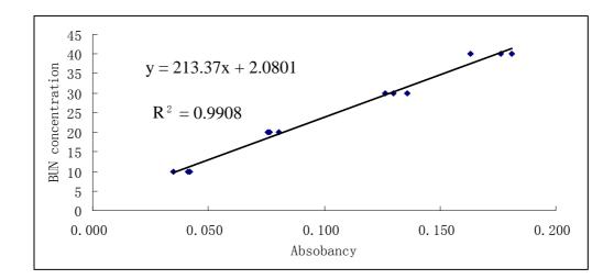
Figure 3.3 The relationship between standard of blood urea nitrogen (BUN) concentration and absorbancy.
