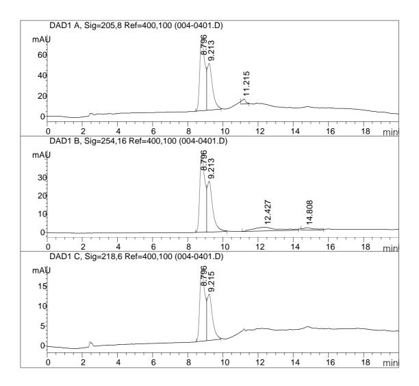
Figure A4 The peak of standard of hypoxanthine.
