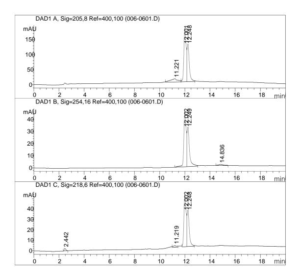
Figure A5 The peak area of standard of xanthine.
