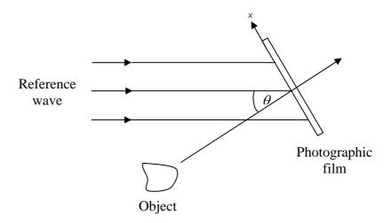
Figure 2.11 Hologram recording with an off-axis reference beam (Hariharan, 1996).
