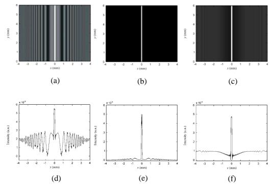
**Figure 3.2** Reconstructed images from the hologram of line object: (a) without modification, (b) with removal of the background, and (c) with removal of the diverging wave. 1-D cross-sectional scans of the corresponding reconstructed images: (d) without modification, (e) with the background removal, and (f) with the diverging wave removal.
