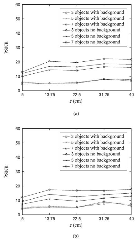
**Figure 4.11** PSNR of image reconstructed from the hologram of multiple line objects having diameter (a) 125  $\mu$ m and (b) 250  $\mu$ m with the separation  $d\xi = 1$  and dz = 1 mm.
