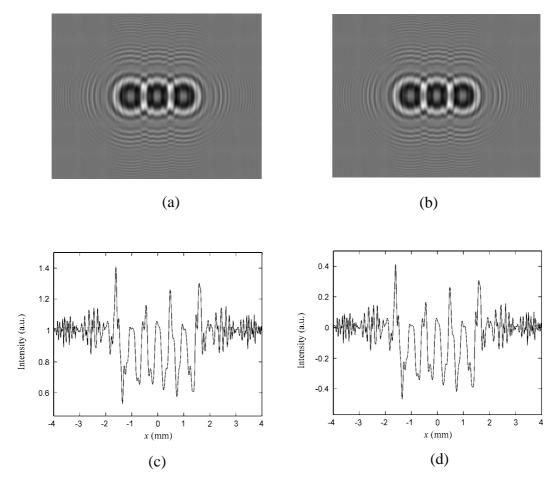
**Figure 4.13** In-line holograms of three square objects: (a) without modification, and (b) with the background removals. 1-D cross sectional scans of: (c) the original hologram, and (d) the modified hologram.
