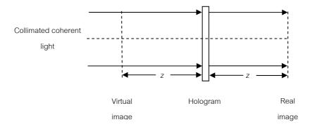
**Figure 2.9** Optical system for image reconstruction from the in-line hologram produces the twin images (Hariharan, 1996).
