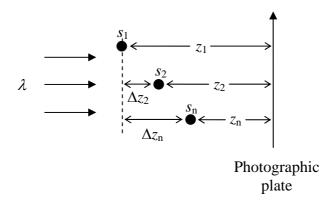
Figure 2.2 Schematic diagram of setup for recording hologram of three objects.
