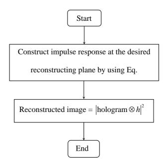
Figure 2.13 Block diagram for computing numerical image reconstruction.
