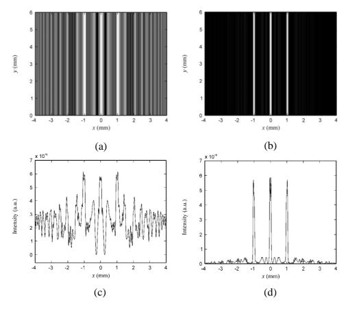
**Figure 4.3** Reconstructed images from the holograms of three line objects: (a) without modification, and (b) with the background removals. 1-D cross-sectional scan of the corresponding images: (c) without modification, and (d) with the background removals.
