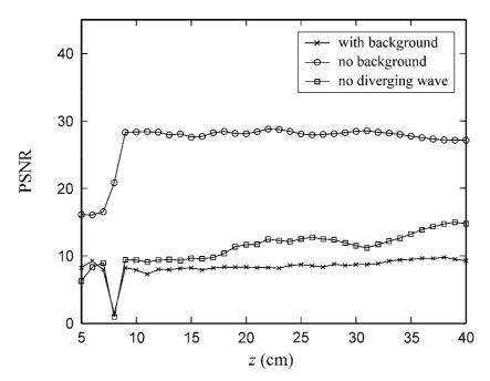
Figure 3.3 PSNR of the image reconstructed from the hologram of a line object with size  $2w = 125 \mu m$  as a function of the recording distance.
