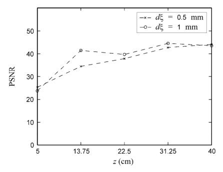
**Figure 4.5** PSNR of images reconstructed from the hologram of 3 line objects having diameter 125  $\mu$ m with the separations  $d\xi = 0.5$  mm and 1 mm as a function of the recording distance.
