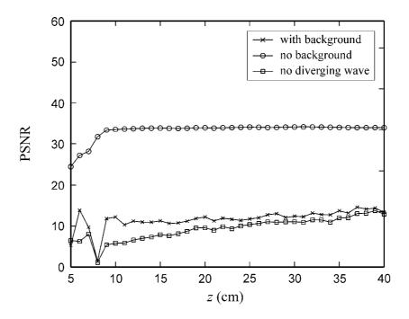
Figure 3.9 PSNR of the image reconstructed from the hologram of a square object with size  $2w = 250 \mu m$  as a function of the recording distance.
