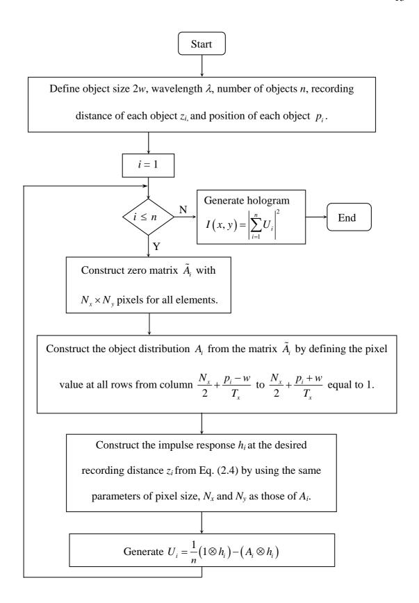
Figure 2.4 Block diagram for simulating hologram of multiple-line object.
