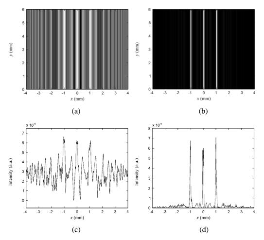
**Figure 4.10** Reconstructed images from the hologram of three line objects: (a) without modification, and (b) with the background removals. 1-D cross sectional scans of the corresponding image: (c) without modification, and (d) with the background removals.
