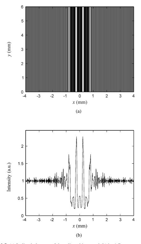
**Figure 2.5** (a) In-line hologram of three line objects and (b) its 1-D cross-sectional scan along the horizontal axis.
