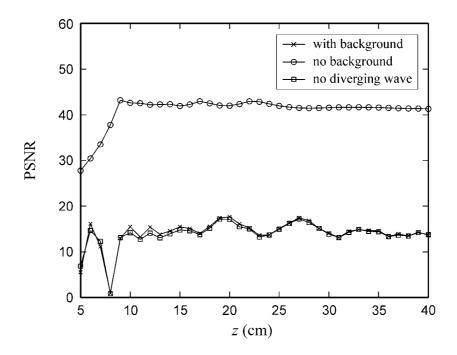
**Figure 3.8** PSNR of the image reconstructed from the hologram of a square object with size  $2w = 125 \mu m$  as a function of the recording distance.
