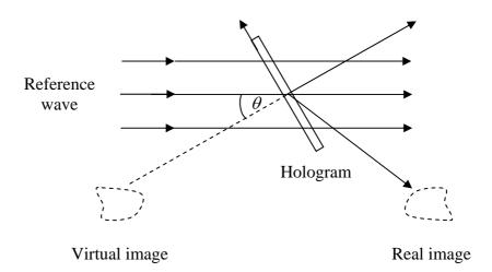
**Figure 2.12** Image reconstruction of a hologram recorded with off-axis reference beam (Hariharan, 1996).
