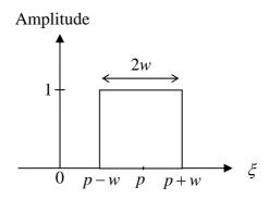
**Figure 2.3** Amplitude distribution function of a line object with size 2w located at a position  $\xi = p$ .
