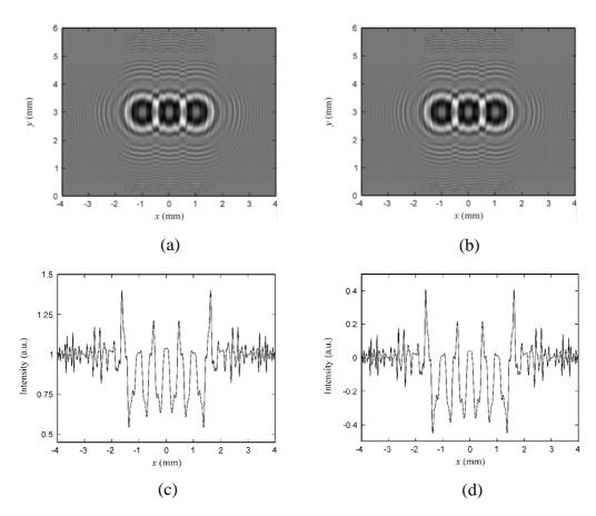
**Figure 4.6** In line holograms of three square objects: (a) without modification, and (b) with the background removals. 1-D cross sectional scans of: (c) the original hologram, and (d) modified hologram.
