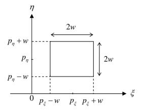
**Figure 2.6** Amplitude distribution function of a square object with size 2w centered at  $\xi = p_{\xi}$  and  $\eta = p_{\eta}$ .
