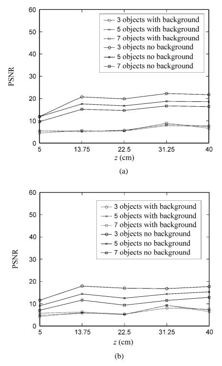
**Figure 4.4** PSNR of images reconstructed from the holograms of multiple line objects having diameter (a) 125  $\mu$ m and (b) 250  $\mu$ m with the separation  $d\xi = 1$  mm and dz = 0 mm.
