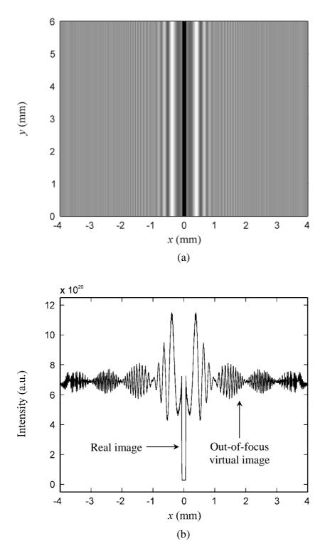
**Figure 2.10** (a) Reconstructed image of a line object and (b) its 1-D cross-sectional scan.
