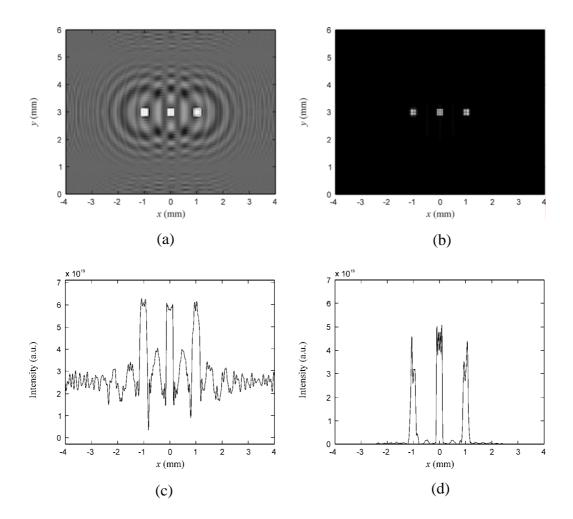
**Figure 4.14** Reconstructed images from the holograms of three square objects: (a) without modification, and (b) with the background removals. 1-D cross-sectional scan of the corresponding images: (c) without modification, and (d) with the background removals.
