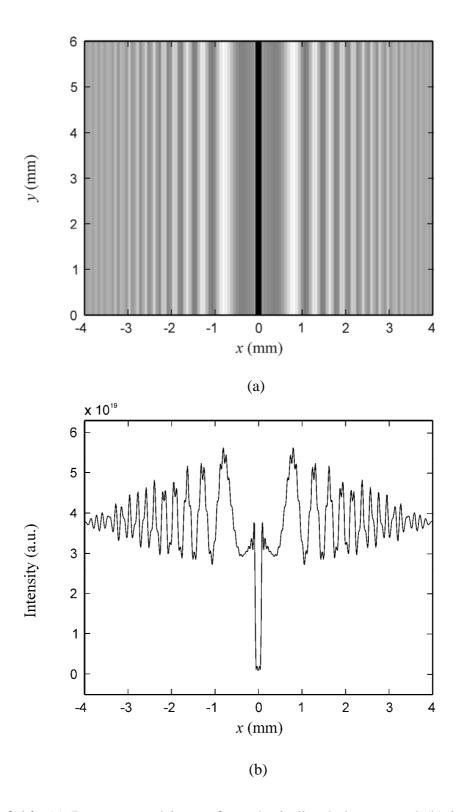
**Figure 2.14** (a) Reconstructed image from the in-line hologram and (b) its 1-D cross-sectional scan.
