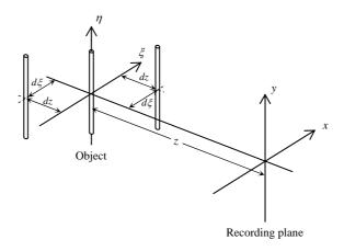
**Figure 4.1** Geometrical distribution of multiple line objects separated by dz and  $d\xi$  along the z and the  $\xi$  directions, respectively.
