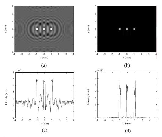
**Figure 4.7** Reconstructed images from the holograms of three square objects: (a) without modification, and (b) with the background removals. 1-D cross-sectional scan of the corresponding images: (c) without modification, and (d) with the background removals.
