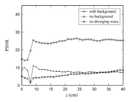
Figure 3.4 PSNR of the image reconstructed from the hologram of a line object with size  $2w = 250 \mu m$  as a function of the recording distance.
