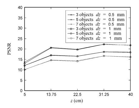
Figure 4.12 PSNR of the image reconstructed from the hologram of multiple line objects having diameter 125  $\mu$ m with the separation dz = 0.5 mm and 1 mm.
