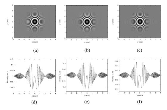
**Figure 3.6** In-line holograms of square object: (a) without modification, (b) with removal of the background, and (c) with removal of the diverging wave. 1-D cross-sectional scans of: (d) original hologram, (e) hologram with removal of the background, and (f) hologram with removal of the diverging wave.
