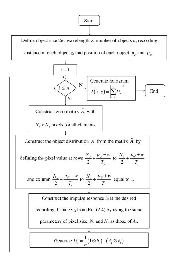
Figure 2.7 Block diagram for simulating hologram of multiple-square object.
