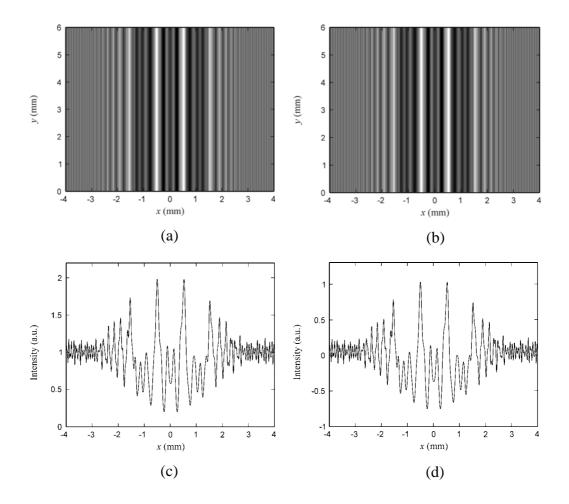
**Figure 4.9** In line holograms of three line objects: (a) without modification, and (b) with the background removals. 1-D cross sectional scans of: (c) the original hologram, and (d) the modified hologram.
