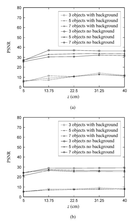
**Figure 4.15** PSNR of image reconstructed from the hologram of multiple square objects having diameter (a) 125  $\mu$ m and (b) 250  $\mu$ m with the separation  $d\xi = 1$  and dz = 1 mm.
