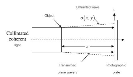
**Figure 2.1** Optical system for recording an in-line (Gabor) hologram (Hariharan, 1996).
