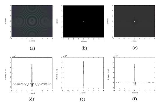
**Figure 3.7** Reconstructed images from the hologram of square object: (a) without modification, (b) with removal of the background, and (c) with removal of the diverging wave. 1-D cross-sectional scans of the corresponding reconstructed images: (d) without modification, (e) with the background removal, and (f) with the diverging wave removal.
