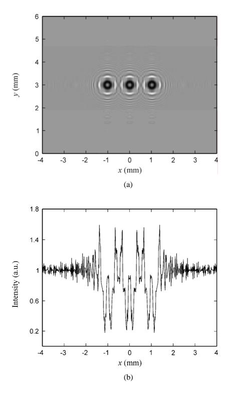
**Figure 2.8** (a) In-line hologram of three square objects and (b) its 1-D cross-sectional scan along the horizontal axis.
