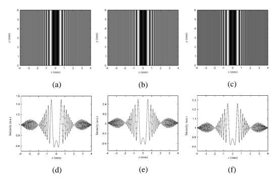
**Figure 3.1** In-line holograms of line object: (a) without modification, (b) with removal of the background, and (c) with the removal of the diverging wave. 1-D cross-sectional scans of: (d) the original hologram, (e) hologram with removal of the background, and (f) hologram with removal of the diverging wave.
