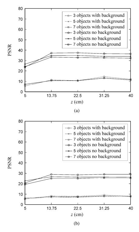
**Figure 4.8** PSNR of images reconstructed from the hologram of multiple square objects having diameter (a) 125  $\mu$ m and (b) 250  $\mu$ m with separation  $d\xi = 1$  mm and dz = 0 mm.
