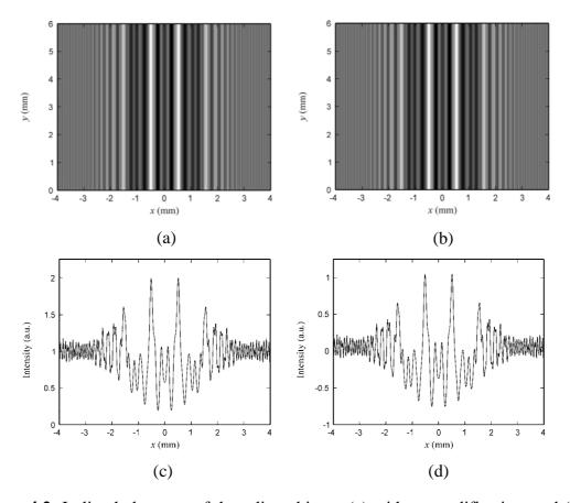
**Figure 4.2** In line holograms of three line objects: (a) without modification, and (b) with the background removals. 1-D cross sectional scans of: (c) original hologram, and (d) modified hologram.
