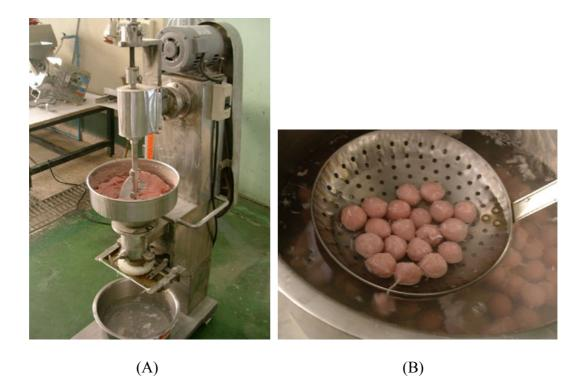
**Figure 2.2** Pork meatball production in pilot-plant scale: (A), pork meatball batter in former machine; (B), pork meatballs after forming in 60 °C water
