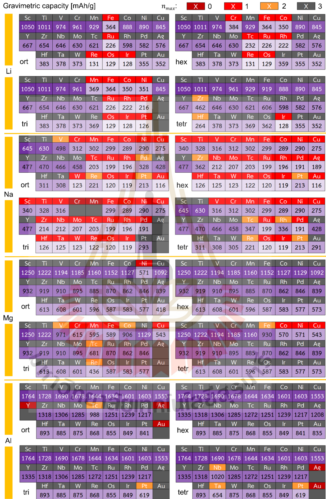
Figure 4.9 Gravimetric capacity and maximum number of adsorption layers ( n_{max} ) for Li, Na, Mg, and Al adsorption on M_2B_2 across different transition metals (M) and phases.
