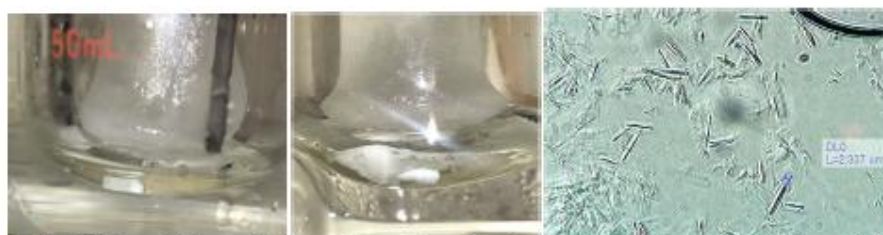
Figure 5. The SFO crystallizer and photomicrographs of papain crystals obtained from SFO crystallization of initial 0.47 g/mL papain solution at -0.5^{\circ}\text{C} .
