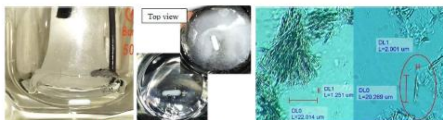
Figure 9. The SFO crystallizer and photomicrographs of papain crystals obtained from SFO crystallization of initial 0.33 g/mL papain solution at -0.5^{\circ}\text{C} .
