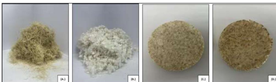
Figure 1. The synthesis process of aerogel mixed with sulfide-modified zero-valent zinc (A.) Raw bagasse (B.) Bagasse after pretreatment (C.) Aerogels from cellulose waste (D.) Aerogel mixed with sulfide-modified zero-valent zinc.
