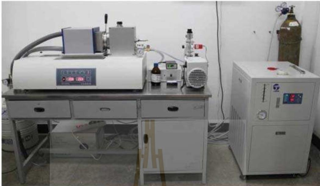
Figure 47 LINSEIS LSR-3 Seebeck type resistivity measurement system.
