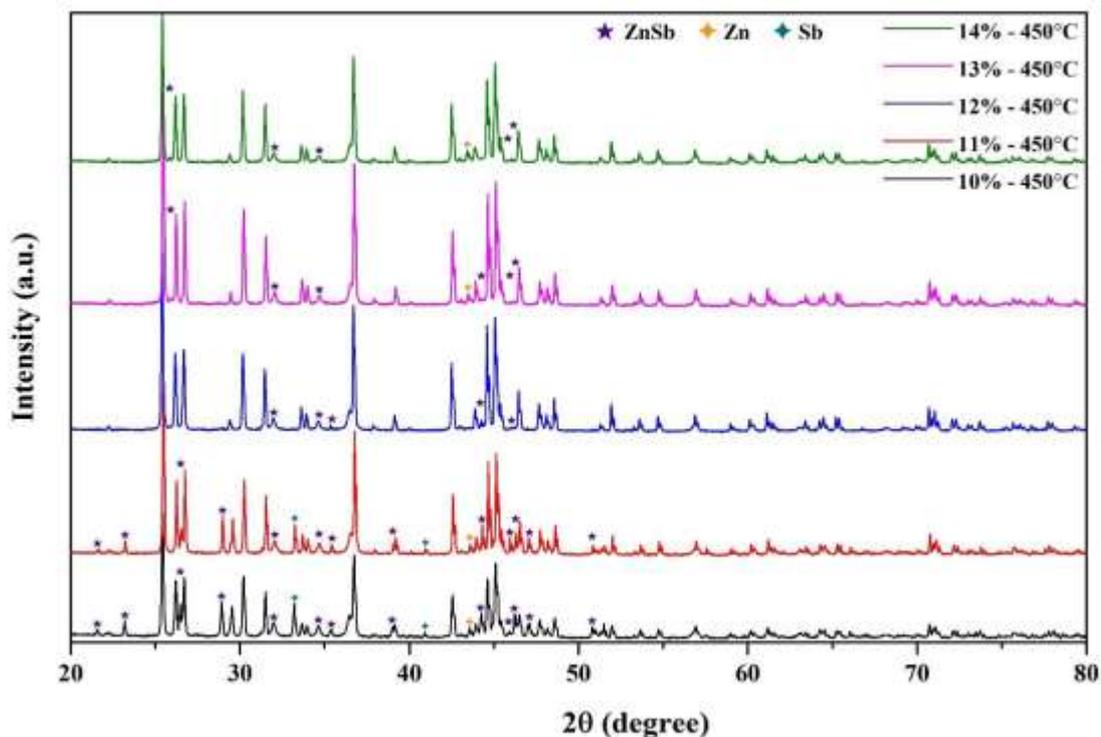
**Figure 53** Comparison XRD pattern of the synthesized  $\beta$ - $\text{Zn}_4\text{Sb}_3$  powders under excessing Zn for 10, 11, 12, 13 and 14 at.% Zn and calcination at 450 °C for 3 hours.
