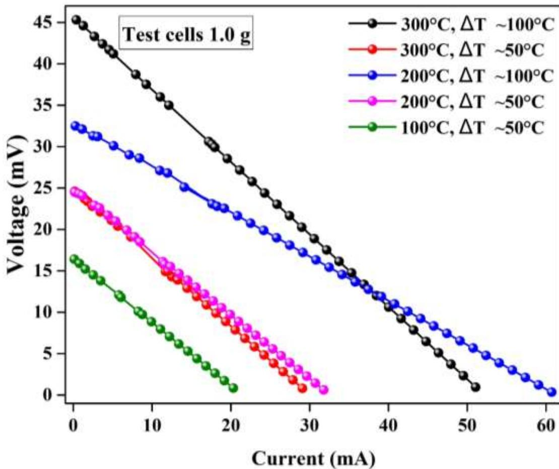
**Figure 64** IV-curve of the test cells of monolithic  $\beta$ -Zn<sub>4</sub>Sb<sub>3</sub>/ZnO TEGs under condition of weight 1.0 g versus different operating  $T_h$  and  $\Delta T$ .
