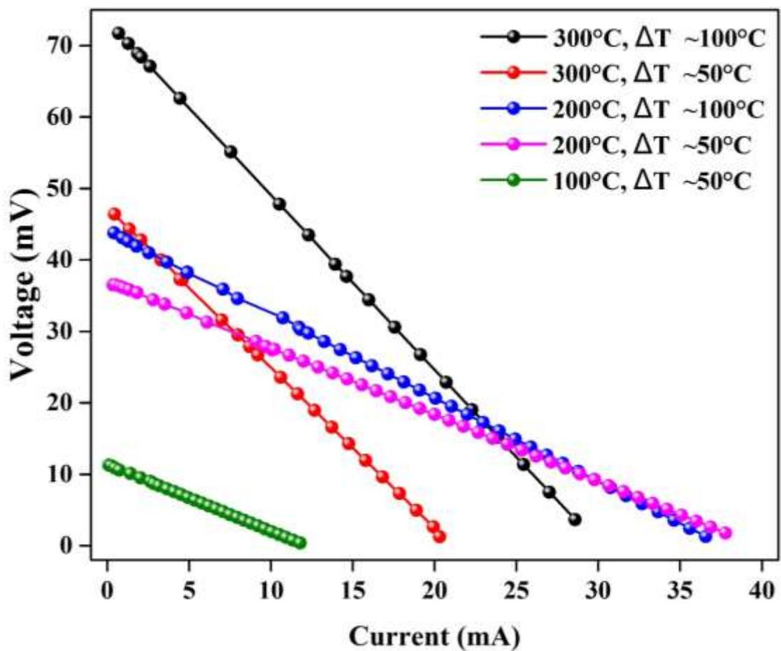
**Figure 66** IV characteristics of the monolithic multi-stack  $\beta$ - $Zn_4Sb_3/ZnO$  TEGs versus varying operation hot side temperature and temperature gradients  $\Delta T$ .
