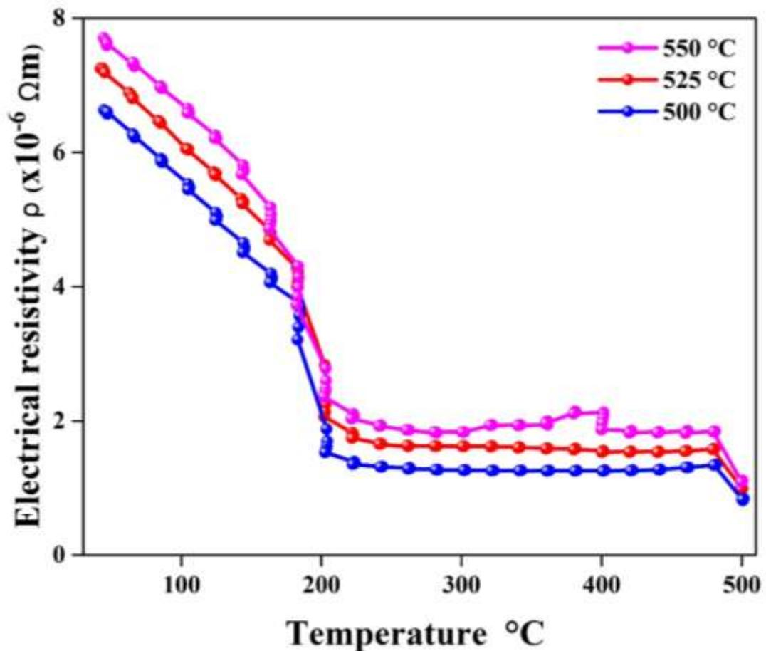
Figure 62 Electrical resistivity of the sintered  $\beta$ -Zn<sub>4</sub>Sb<sub>3</sub> pellets versus varying temperature.
