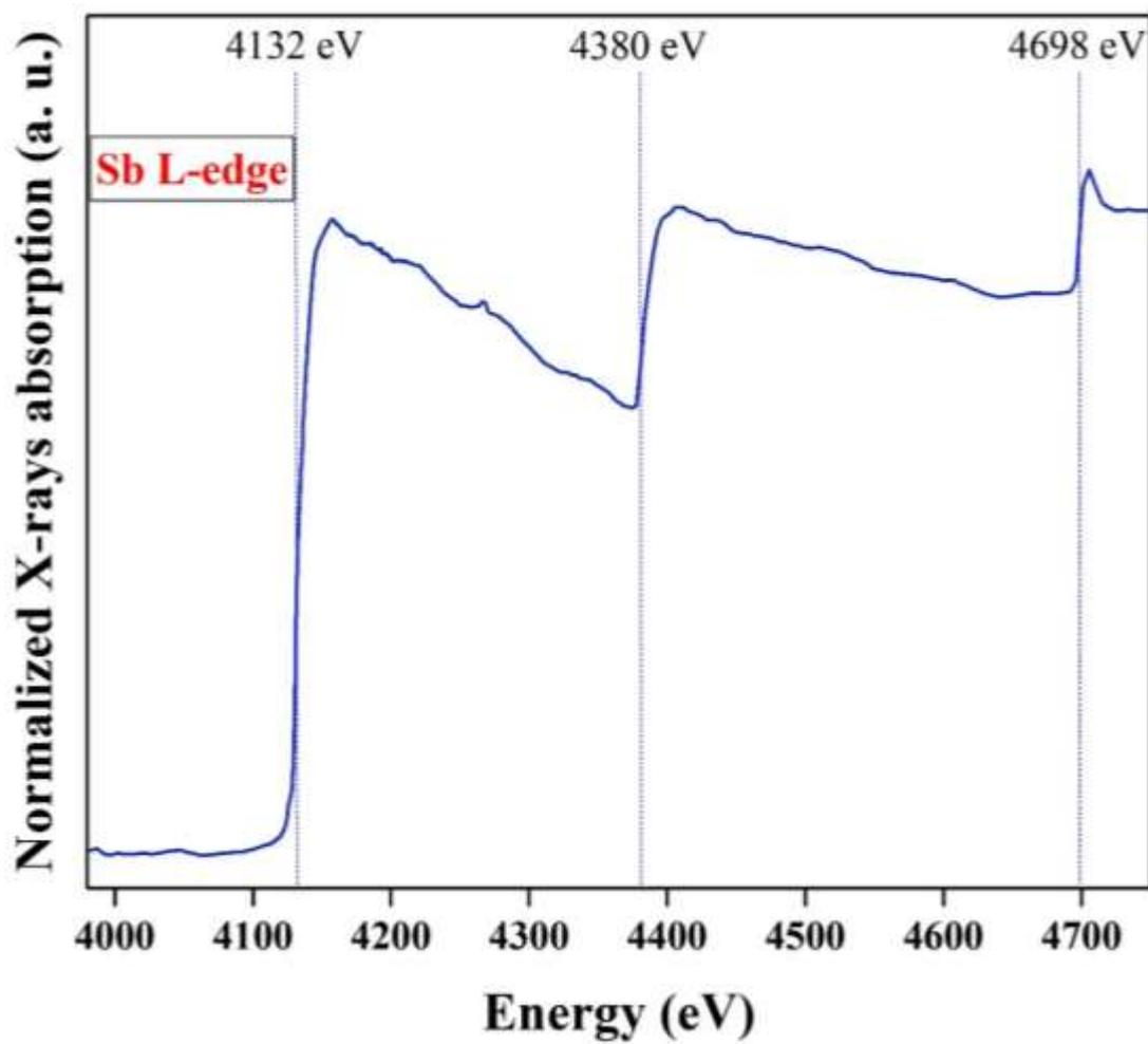
Figure 59 Normalized XANES of Sb L3, L2 and L1-edge of the high pure synthesized  $\beta$ -Zn<sub>4</sub>Sb<sub>3</sub> powder.
