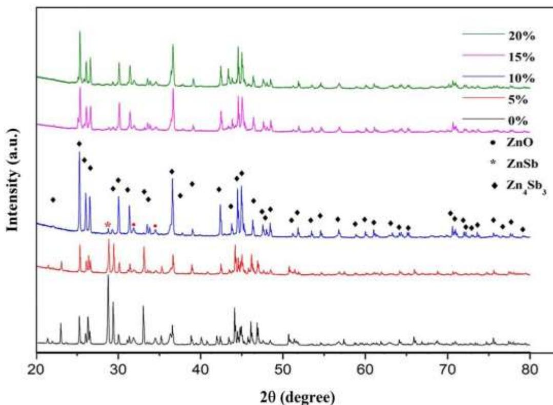
**Figure 50** The comparison XRD pattern of the synthesized  $\beta$ -Zn<sub>4</sub>Sb<sub>3</sub> powders under varying excessed Zn condition via calcination temperature 400 °C and held for 3 hours.
