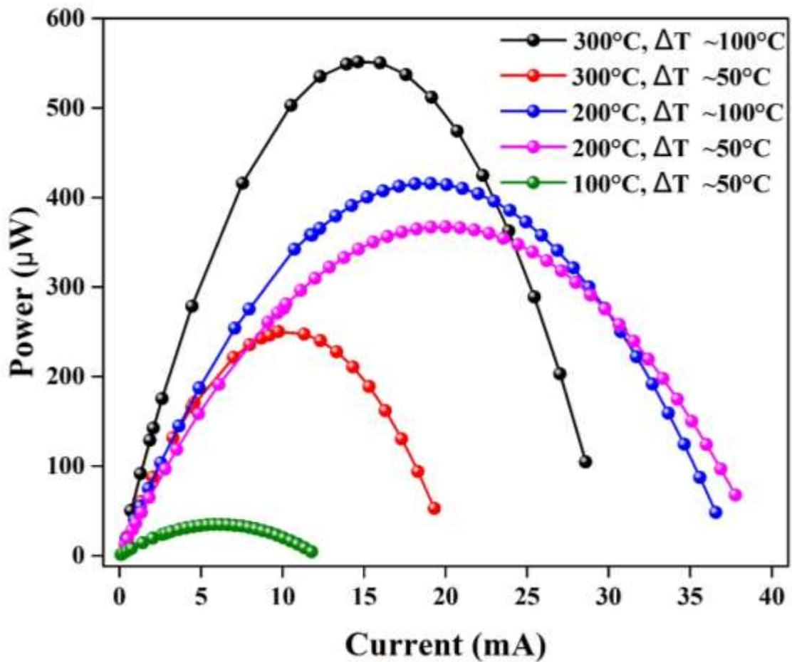
Figure 67 Electrical power output curves of the monolithic multi-stack  $\beta$ - $\text{Zn}_4\text{Sb}_3/\text{ZnO}$  TEGs versus varying operation hot side temperature and temperature gradients  $\Delta T$ .
