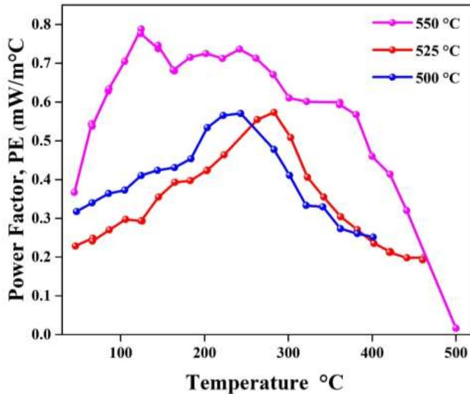
Figure 63 Electrical power factor of the sintered  $\beta$ -Zn<sub>4</sub>Sb<sub>3</sub> pellets versus varying temperature.
