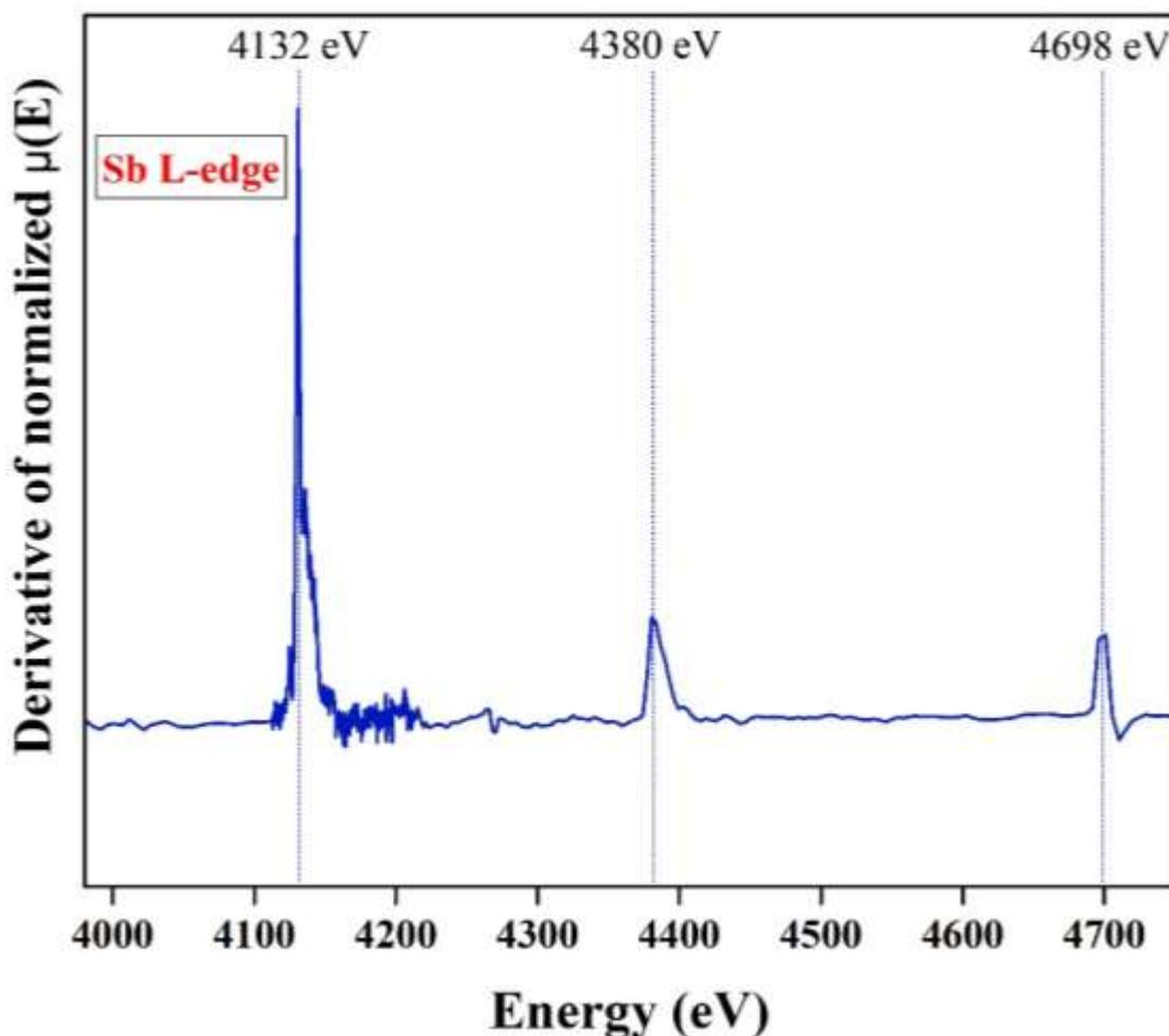
**Figure 60** Derivative normalized XANES of Sb L3, L2 and L1-edge of the high pure synthesized  $\beta$ -Zn<sub>4</sub>Sb<sub>3</sub> powder.
