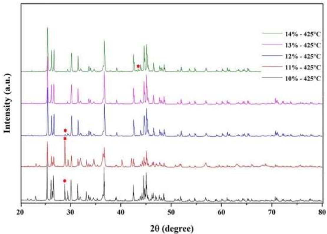
Figure 55 Comparison XRD pattern of the synthesized  $\beta$ - $\text{Zn}_4\text{Sb}_3$  powders under excessing Zn for 10, 11, 12, 13 and 14 at.% Zn and calcination at 425 °C for 3 hours.
