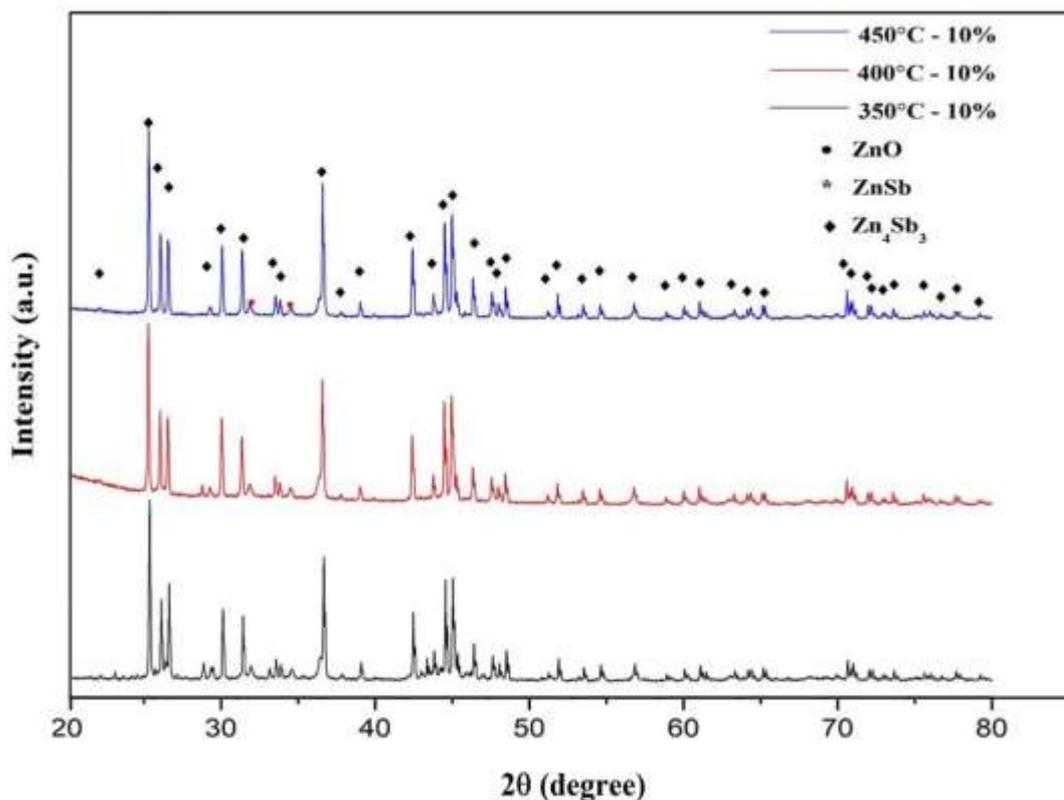
**Figure 52** The comparison XRD pattern of the synthesized  $\beta$ - $\text{Zn}_4\text{Sb}_3$  powders under varying calcination temperature at 350 °C, 400 °C and 450 °C via adding 10 at.% Zn and calcination holding time for 3 hour.
