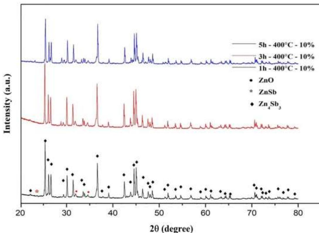
**Figure 51** XRD pattern of varying holding time via excessing Zn of 10 at.% Zn and calcination temperature 400 °C.
