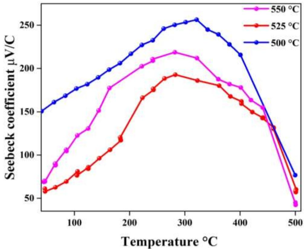
**Figure 61** Seebeck coefficient of the sintered  $\beta$ - $\text{Zn}_4\text{Sb}_3$  pellets versus varying temperature.
