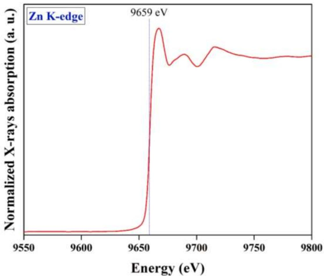
Figure 57 Normalized XANES of Zn K-edge of the high pure synthesized  $\beta$ - $\text{Zn}_4\text{Sb}_3$  powder.
