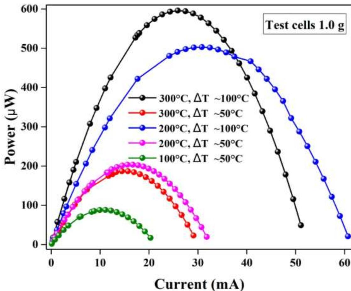
Figure 65 Electrical power output curves of the test cells of monolithic  $\beta\text{-Zn}_4\text{Sb}_3/\text{ZnO}$  TEG module under condition of weight 1.0 g versus different operating  $T_h$  and  $\Delta T$ .
