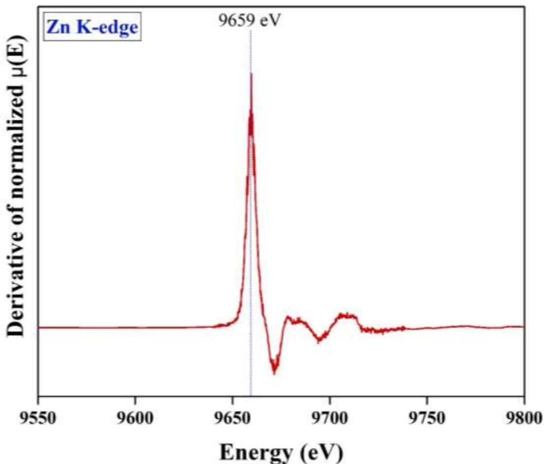
Figure 58 Derivative normalized XANES of Zn K-edge of the high pure synthesized  $\beta$ - $\text{Zn}_4\text{Sb}_3$  powder.
