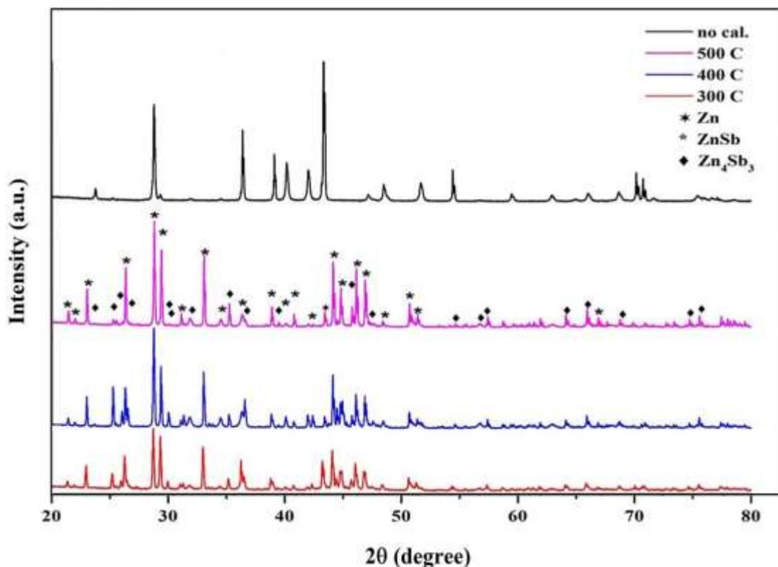
**Figure 49** X-ray diffraction patterns of the synthesized  $\beta$ - $Zn_4Sb_3$  powders under conditions of calcination temperature non-calcined, 300 °C, 400 °C and 500 °C without excess of Zn.
