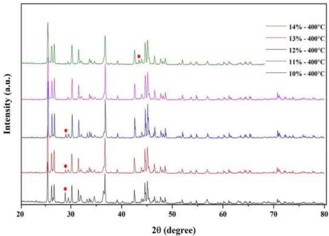
Figure 54 Comparison XRD pattern of the synthesized  $\beta$ - $\text{Zn}_4\text{Sb}_3$  powders under excessing Zn for 10, 11, 12, 13 and 14 at.% Zn and calcination at 400 °C for 3 hours.
