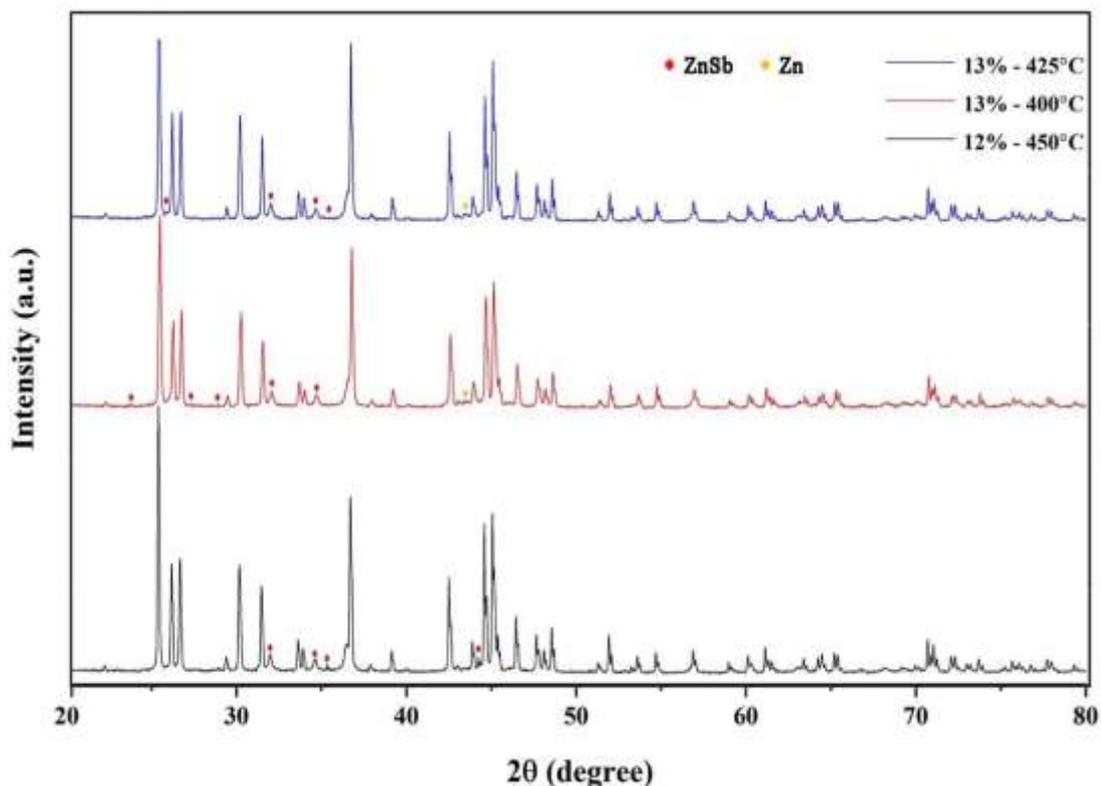
**Figure 56** Comparison of the synthesis series of excessing Zn for 10, 11, 12, 13, 14 and 15 at.% Zn and calcination at 400 °C, 425 °C, 450 °C for 3 hours.
